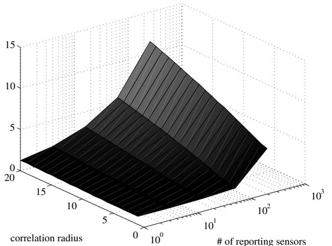
Fig. 2. Precision (inverse sum-variance) for uniform multiresolution sampling (as in Figure 1) as a function of correlation radius (for a minimum correlation value of 0.1) and number of reporting sensors; here the prior data uncertainty and measurement noise are  $\sigma_x = 1$  and  $\sigma = 1/4$  respectively.
