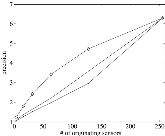
Fig. 4. Relative precision for PROSE for  $\mu = 1$  ( $\diamond$ ) and  $\mu = 0$  ( $\times$ ). Precision for multiresolution sampling is shown as a solid line for comparison. The correlation radius is 5 (for a minimum correlation of 0.1); prior data uncertainty and measurement noise are the same as in Figure 1.
