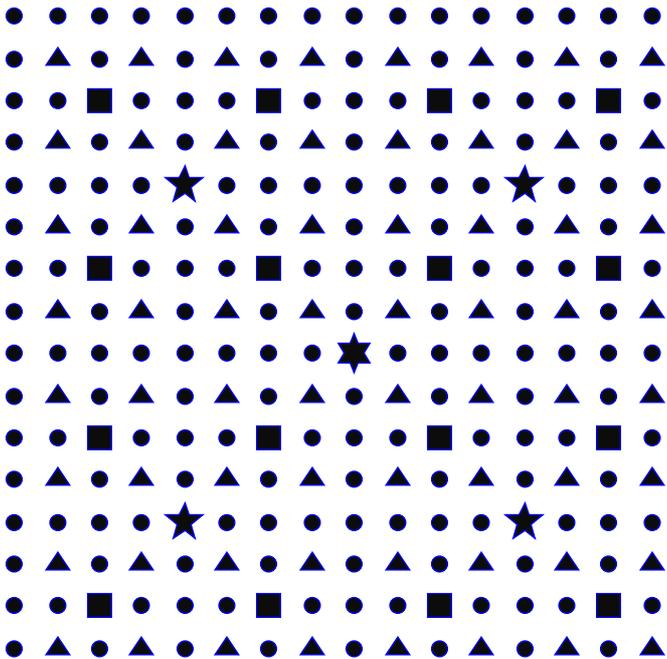
Fig. 1. Two-dimensional multiresolution grid of 256 sensors. Sensor nodes are represented by polygons, with fewer sides as the spatial sampling rate increases. The 6-pointed star denotes the central server. At level  $L = \log_4 256$ , all nodes sample the field.
